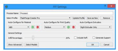
• **Auto-Configure for Print Quality**: Adjusts layer height, infill density, and other quality settings based on the level you desire.
